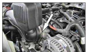
5. Loosen the hose clamps that secure the intake tube to the throttle body and air filter housing. Unhook the radiator hose clip from the intake tube and then remove the intake tube from the vehicle.
