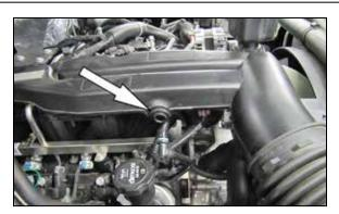
4. Disconnect the crank case vent hose from the intake tube plenum as shown.
