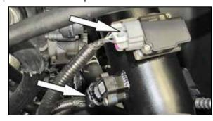
20. Reconnect the mass air sensor and humidity sensor electrical connections.
