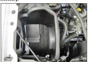
11. Install the heat shield assembly onto the air filter housing mounting plate location and secure with three of the factory bolts from step #8.
