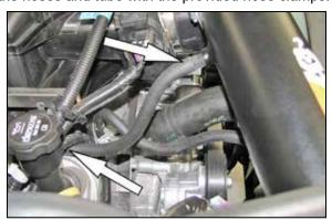
18. Install the provided crank case vent hose onto the fitting installed into the K&N® intake tube and then onto the valve cover port. Secure the hose to the valve cover port with the provided hose clamp.
