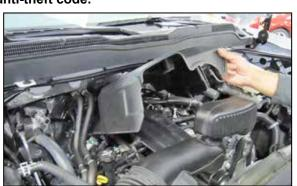
2. Lift up and remove the engine cover from the engine.
