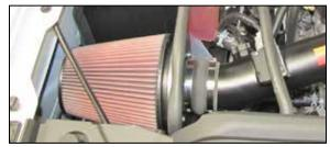
19. Install the K&N<sup>®</sup> air filter and secure with the provided hose clamp.
