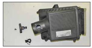
12. Remove the screws securing the mass air sensor and humidity sensors into the air filter housing and then remove the sensors.
