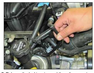
7. Release the locking ring and then disconnect the crank case vent tube from the valve cover vent port.
