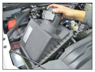
6. Lift up the air box to dislodge it from the mounting grommets, and then remove it from the vehicle as shown.
