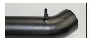
14. Install the provided vent fitting into the K&N® intake tube as shown.
