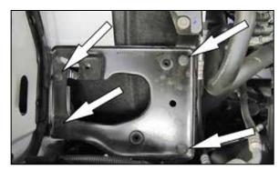
8. Remove the four bolts that secure the air filter mounting tray to the inner fender and then remove the tray.
