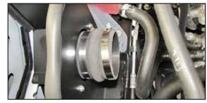
15. Install the provided coupling hose (08699) onto the filter adapter and secure with the provided hose clamp.
